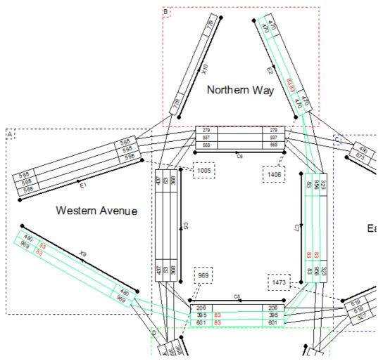
Figure 4.19: Lane Flow Components for Traffic from Zones B to A
