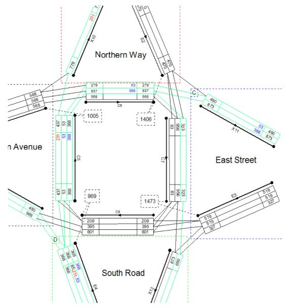
Figure 4.18 - Lane Flow Components for Traffic from Zone D
